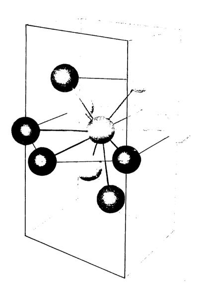
Fig. 2. A portion of the unit cell illustrating the tenfold coordination. Relative to Figure 1, the origin of the unit cell has been displaced by (0 0 1/2).
